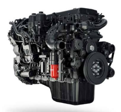
Power range Up to 500 kW Torque Up to 2850 Nm Engine model XCURSOR 13 (6 Cyl., 12.9 litres) Exhaust System Hi-eSCR2
